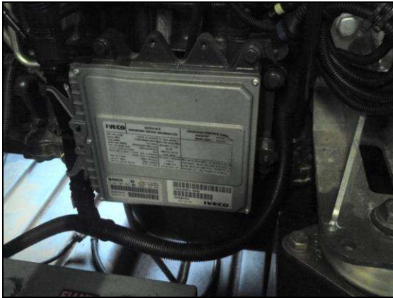
Iveco EDC62 mounted on the engine
