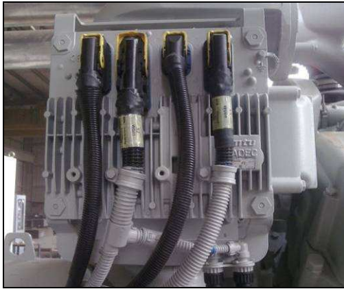
ADEC ECU Mounted on the engine
